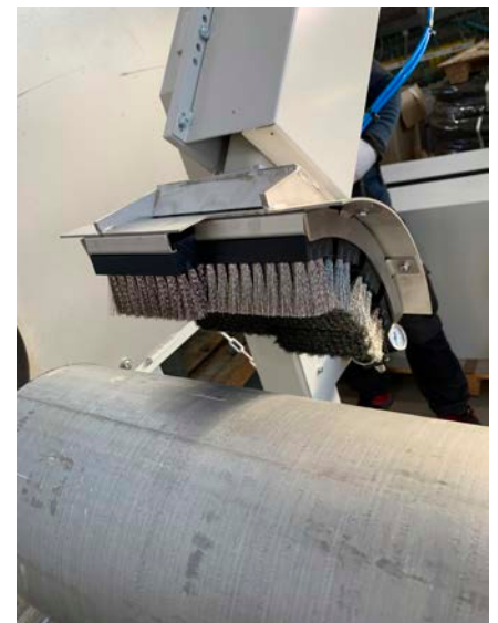
Figure 3: Log cleaning system (Source: extrutec)
